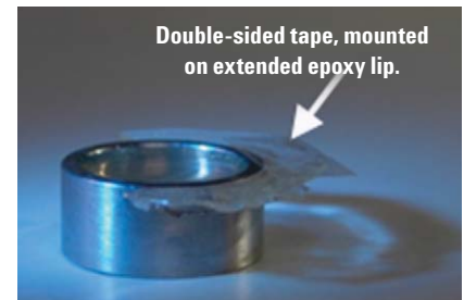
Figure 2. Gel sample, ready for testing in inverted NanoVision puck with extended epoxy lip.
