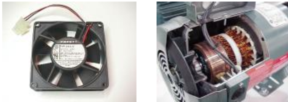
Two examples of DC motors – the picture on the right is cut open to show the windings. You can find more information on motors at http://my.execpc.com/~rheadley/magmotor.htm
