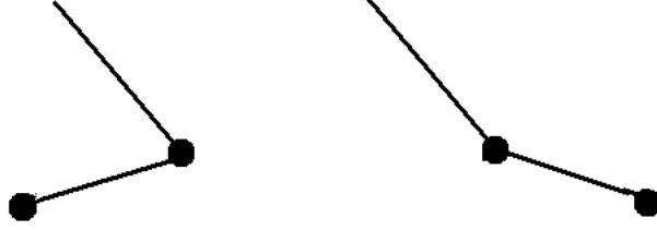
Figure 3.8: Normal modes related to the stable equilibrium of the double pendulum.
