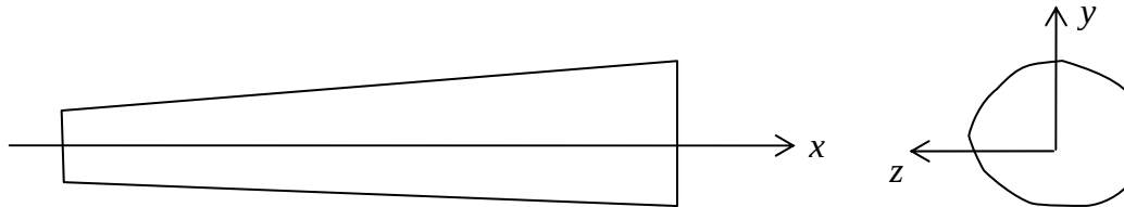
Figure 4.3.1: A slender straight component; (a) longitudinal axis, (b) cross-section
