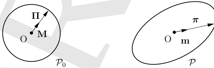
Figure 3.14: Spatially homogeneous deformation of a sphere.
