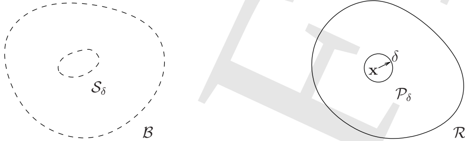
Figure 4.3: A limiting process used to define the mass density \rho at a point \mathbf{x} in the current configuration.
