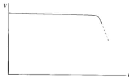
Fig. 7-2. Typical curve of output voltage as a function of output current for a commercial voltage-stabilized power supply.
