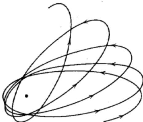
Fig. 12-1. Orbits for a potential that does not have the exact 1/r form do not close upon themselves and precess as shown here. The orbits remain planar as long as the potential is radial.
