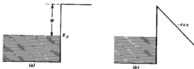
Fig. 5-9. (a) Electronic energy levels in metal. E_F is the Fermi energy and W is the work function. (b) Potential altered by an external electric field.
