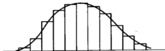
Fig. 5-8. Approximation of smooth barrier by a juxtaposition of square potential barriers.
